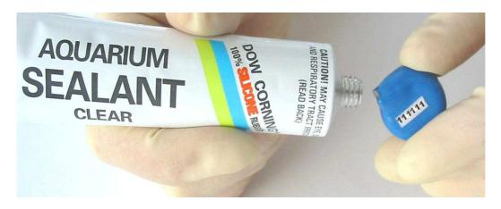
Silicone should be allowed to dry overnight at room temperature OR for 2 hours at 40 ℃
